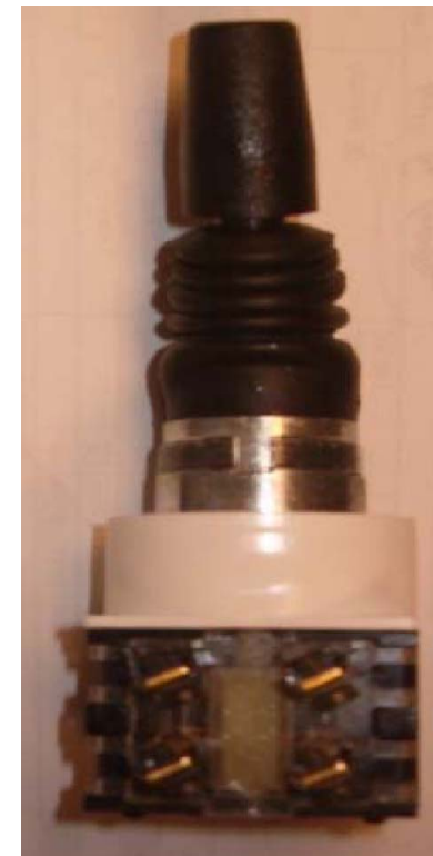
The front view of the switch is shown in the picture. There are 4 terminals on each side.
